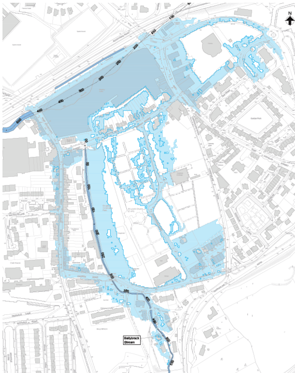
Figure 12.6: Extract from the Douglas FRS Flood Map showing the 1 in 100 year fluvial flood extent.
